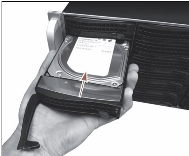
Figure 209 Install the drive into the BlackPearl Storage Manager.
