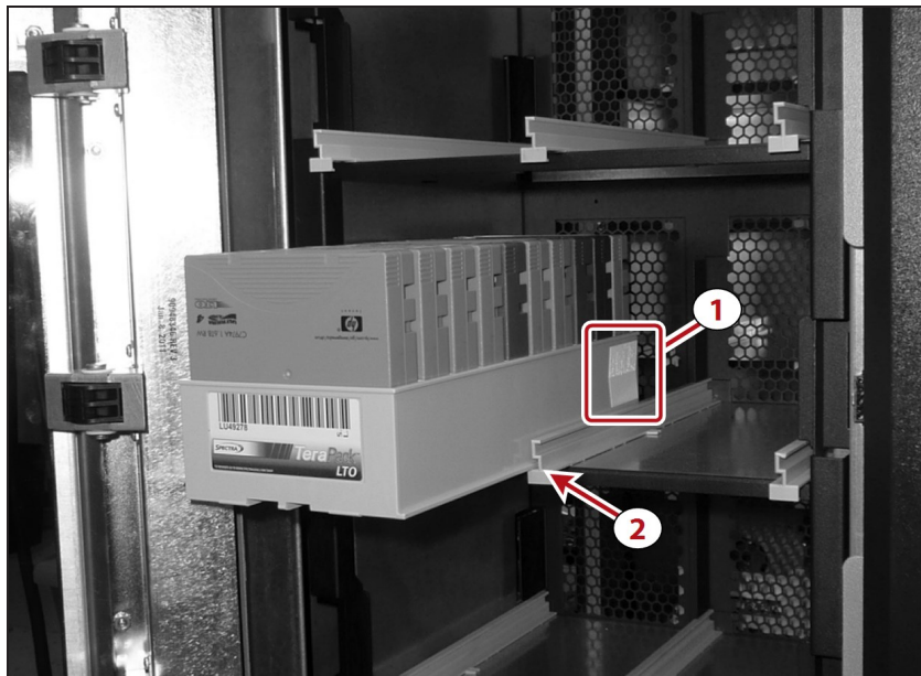
Figure 239 Insert the magazine into the bulk TAP carousel, making sure that it is correctly positioned.
