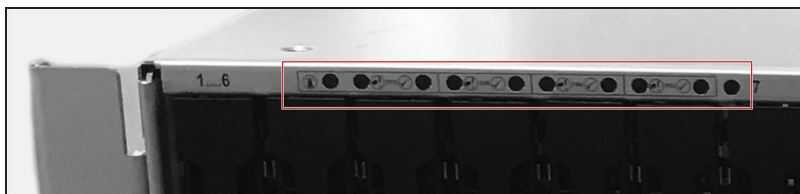
Figure 163 The top left section of the front of the Gen2 X chassis (front bezel removed) showing system status LEDs.
