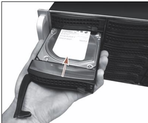
Figure 136 Install the drive into the BlackPearl NAS.
