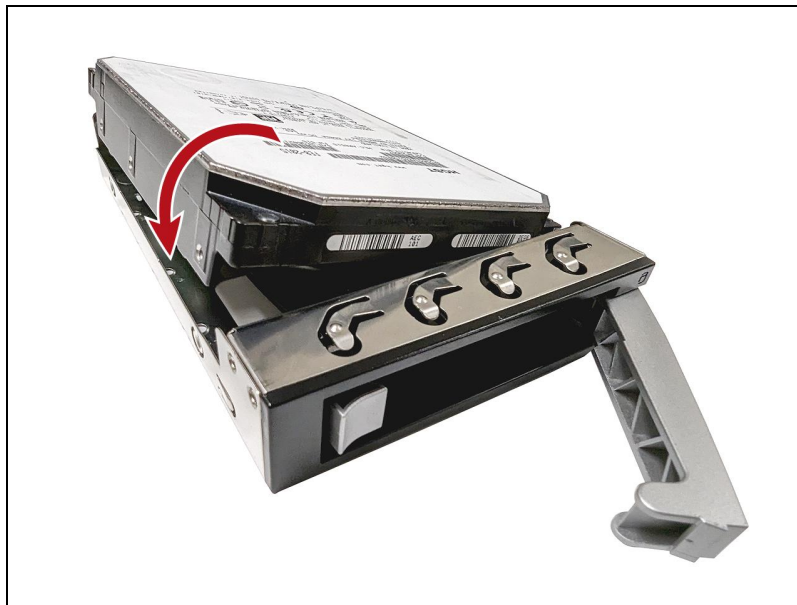
Figure 114 Insert drive into chassis.
