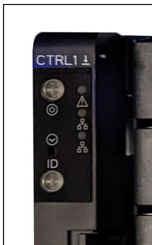
Figure 93 The Gen3 H Series chassis system status LEDs.
